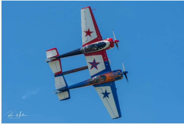
Yak 110 – two Yak-55s joined at wing center section with jet engine mounted on center line. Taken at Fargo AirSho, Fargo, ND
