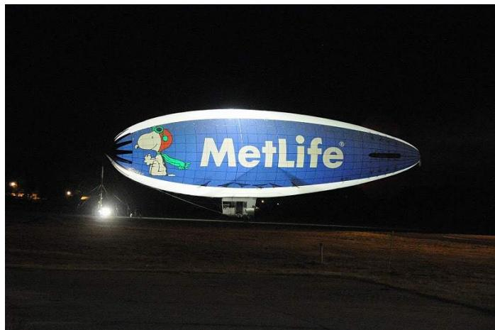
Helium that fills the lifting envelope is inside what you see on the outside. What is outside is pressurized air supplied by small blowers. This air envelope outside the helium envelope, is pressurized from the engines during flight. When moored to its standard, as you can see in these pictures, portable electric blowers are used to keep the pressure inside that air envelope. A full set of generators is used to provide power for the blowers and the lights while on the ground.
